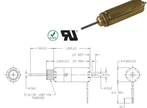
Solenoid shown energized with plunger fully seated in extended position Supplied with mounting bracket, hex nut and lock washer shipped loose
