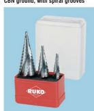
The deep-ground, spiral cutting groove offers absolutely smooth running and high cutting performance. In particular, swarf which does not break off is carried away cleanly, as with a spiral drill. This reduces the formation of cutting build-up and cold welding on the cutting edges. The cone makes pulling back easier from metal sheets that have been drilled through.
