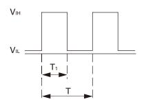
$$V_{IH} = 4.75 \text{ to } 5.25 \text{ V} \quad V_{IL} = 0 \text{ to } 0.4 \text{ V}$$
