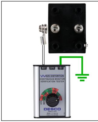
Figure 5. Connecting the Wave Distortion Monitor Verification Tester to the Mini Monitor's 10mm mat snap
