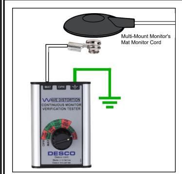
Figure 7. Connecting the Wave Distortion Monitor Verification Tester to the Multi-Mount Monitor's mat monitor cord
