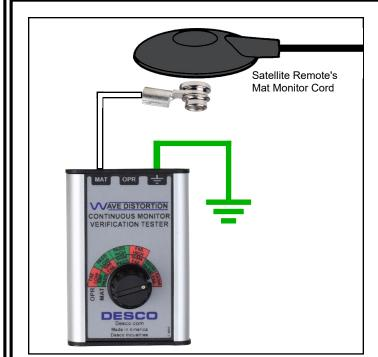
Figure 9. Connecting the Wave Distortion Monitor Verification Tester to the satellite remote's mat monitor cord
