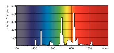
LDPB\_PLL4P\_830-Spectral power distribution B/W
