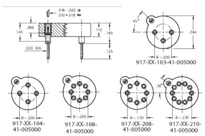
**Description:** Transistor TO Socket Through-Hole Mount
