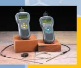
$\pm$  0.005 °C and 0.001 °C resolution. They accept inputs from RTDs or thermistors and with Hart's
