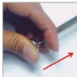
Push the plunger of pin extractor
