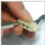
Put the pin extractor into housing
