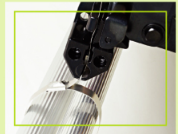
Tensioning and cutting off stainless steel cable ties
