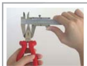
Outside diameter measurement
