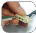
Put the pin extractor into housing
