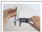
Inside diameter measurement
