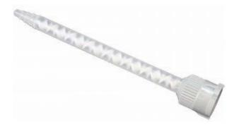
The 8MT Mixing Tips are single use static mixer for 2-part low to medium viscosity cartridge systems. The mixer works using stationary elements inside a narrow cylindrical tube. This forces the materials to combine as it travels through the length of the mixer and provides a homogenous mix of hardener and resin that can be applied directly onto the targeted area.
