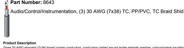
Three 30 AWG stranded (7x38) tinned copper conductors, conductors cabled around textile strength member, polpyropylene insulation, tinned copper braid shield (95% shield coverage), PVC jacket.
