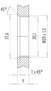
Installation direction: o-ring sits on chamfer.
