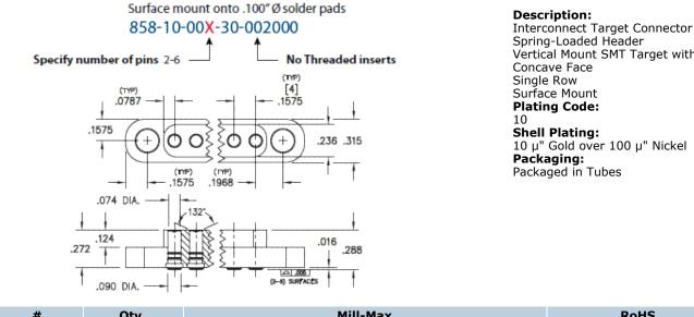
Spring-Loaded Header Vertical Mount SMT Target with Concave Face Single Row Surface Mount Plating Code: Shell Plating: 10 µ" Gold over 100 µ" Nickel Packaging:
