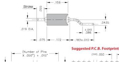
Interconnect SLC Header Spring-Loaded Header Horizontal Mount Single Row Surface Mount Plating Code: 22 Shell Plating: 20µ" Gold over 100µ" Nickel Inner Spring Plating: 10µ" Gold
