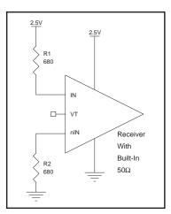
Figure 4A. Unused Input Handling
