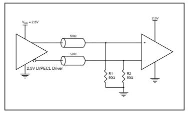
Figure 6C. 2.5V LVPECL Driver Termination Example
