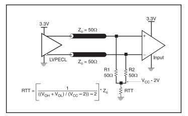
Figure 5A. 3.3V LVPECL Output Termination
