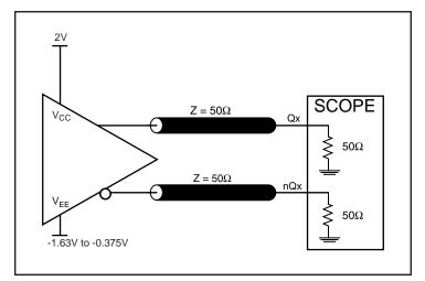
**Output Load AC Test Circuit**
