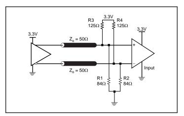
Figure 5B. 3.3V LVPECL Output Termination
