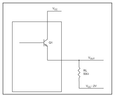
Figure 8. LVPECL Driver Circuit and Termination
