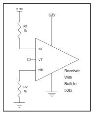
Figure 4B. Unused Input Handling
