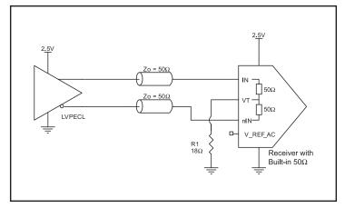
Figure 3B. IN/nIN Input with Built-In 50 $\Omega$  Driven by an LVPECL Driver
