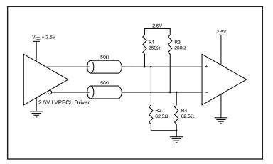
Figure 6A. 2.5V LVPECL Driver Termination Example
