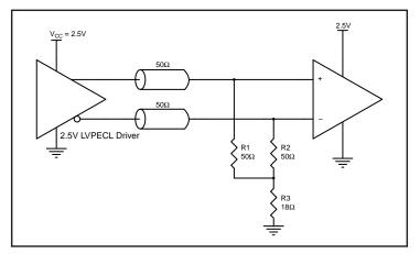
Figure 6B. 2.5V LVPECL Driver Termination Example
