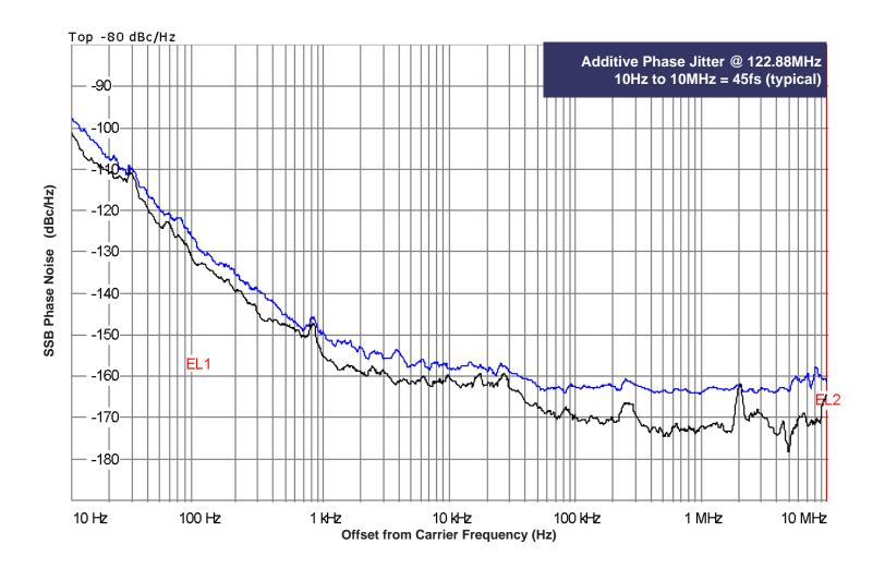
As with most timing specifications, phase noise measurements has issues relating to the limitations of the equipment. Often the noise floor of the equipment is higher than the noise floor of the device. This is illustrated above. The device meets the noise floor of what is shown, but can actually be lower. The phase noise is dependent on the input source and measurement equipment. The source generator used is, low noise Wenzel Oscillator at 122.88MHz.
