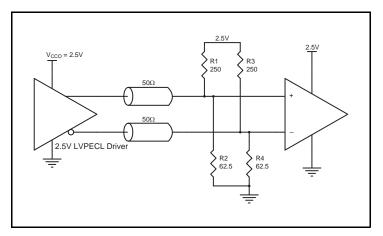
Figure 5A. 2.5V LVPECL Driver Termination Example
