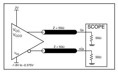
**LVPECL Output Load AC Test Circuit**
