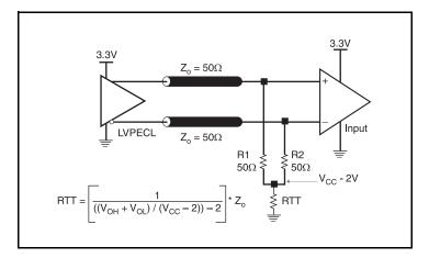
Figure 4A. 3.3V LVPECL Output Termination
