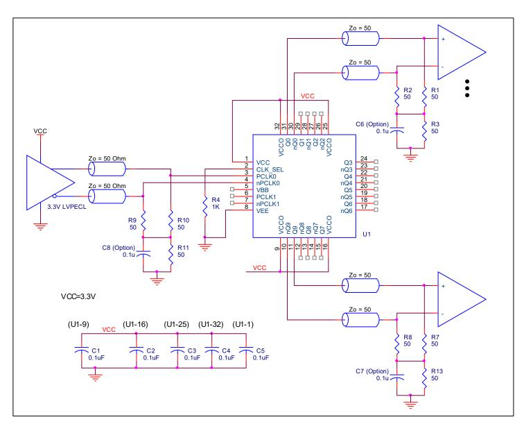
Figure 8. 853S111B Example LVPECL Clock Output Buffer Schematic
