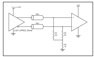
Figure 5B. 2.5V LVPECL Driver Termination Example
