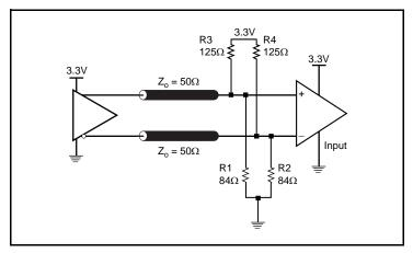
Figure 4B. 3.3V LVPECL Output Termination
