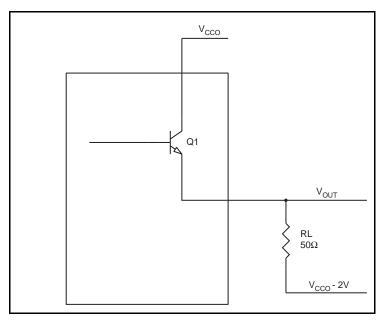
Figure 9. LVPECL Driver Circuit and Termination
