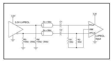
Figure 3D. PCLK/nPCLK Input Driven by a 3.3V LVPECL Driver with AC Couple
