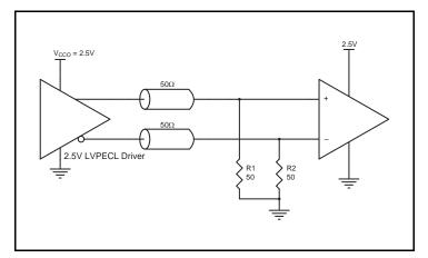
Figure 5C. 2.5V LVPECL Driver Termination Example
