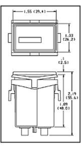
\* Panel cutout dimensions are  $\pm$  .010 tolerance All dimensions shown in inches and (metric)
