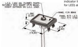
PANEL INSERT WITH HOLE FOR LED
