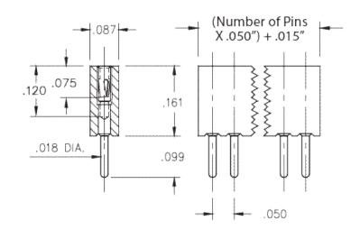
**Description:** Interconnect Socket Standard Solder Tail Socket Accepts .015"- .020" (0,38 - 0,508 mm) dia leads Single Row Through Hole Plating Code: 43 Shell Plating: 200 µ" Tin (matte finish) over 100 µ" Nickel Inner Contact Plating:
