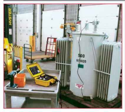
The DTR\* Model 8510 is a portable digital transformer ratiometer designed for on-site testing of power, potential and current transformers. When connected to a non-energized transformer, the DTR\* accurately measures primary to secondary turns ratio, while simultaneously displaying polarity and excitation current.
