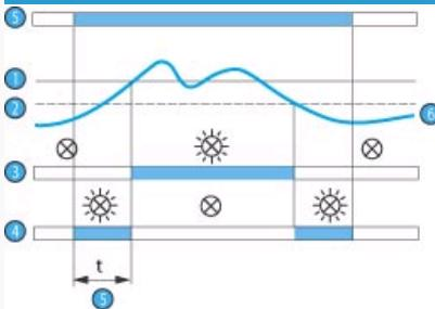
The MIC relay controls the overcurrent. The relay closes when the current exceeds the threshold displayed on the front face and opens when it falls below the threshold minus the hysteresis. When terminal Y1 is connected to A1 (+), the output is inverted. The relay opens when the current exceeds the threshold displayed on the front face and closes again when it falls back below the hysteresis (undercurrent).
