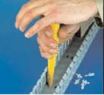
Panel Mounting Rivets and Tool: WAGO Wire-Way panel rivets are one piece drive rivets that provide a fast, economical means of affixing wiring duct. The rivet is inserted into a 3/16" pre-punched hole and the pin is driven into the base, thereby expanding the rivet legs and locking the duct and sub-panel in place. The panel thickness (including the duct thickness) should be a maximum of 3/16". A panel rivet tool is also available for quick and easy installation of the drive rivets.
