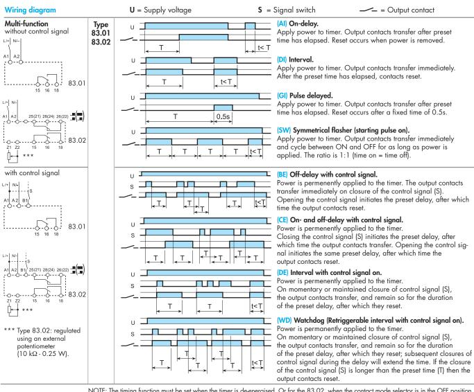
NOTE: The timing function must be set when the timer is de-energised. Or for the 83.02, when the contact mode selector is in the OFF position.
