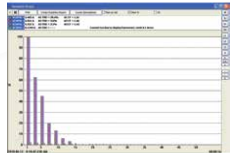
Display all harmonics from 1 st to 50 th in bargraph form for voltage, current and power.
