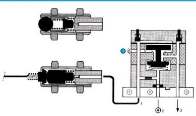
Supplied at industrial pressure, the relay produces a permanent bleed at its input port. A sensor shutting off this bleed causes the relay to switch.
