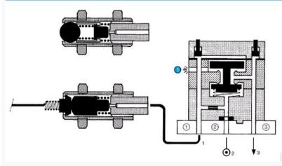
Supplied at industrial pressure, the relay produces a permanent bleed at its input port. A sensor shutting off this bleed causes the relay to switch.
