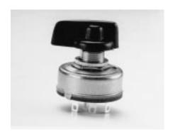
The 800-Series rotary switches are single pole and AC rated to 6 amps. These switches feature a self-cleaning wiping action and a silver-plated contact system. A nylon actuator and shaft in a metal clad package highlight the construction of this multi-position switch.
