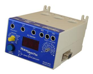
The Model 777-P2 Series is a family of fully programmable electronic overload relays. They are designed to monitor and protect any 3-phase 200-480VAC (500-600VAC for 777-575-P2) motor drawing 2-800 full load amps (external CTs are required above 90 amps). They provide unsurpassed protection from faulty voltage, underload and overload conditions. Common applications include conveyor systems, HVAC equipment, saws and grinders, fan motors and almost any pumping application.
