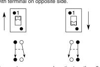
To create common poles, tie together 2 adjoining terminals on 1 (either) side of switch.
