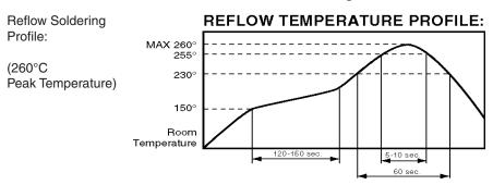
WAVE SOLDERING: 260°C maximum solder temperature for 5 seconds max.
