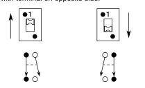
To create common poles, tie together 2 adjoining terminals on 1 (either) side of switch.
