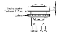
Maximum panel thickness 4 Mounting hole size Ø22.5
