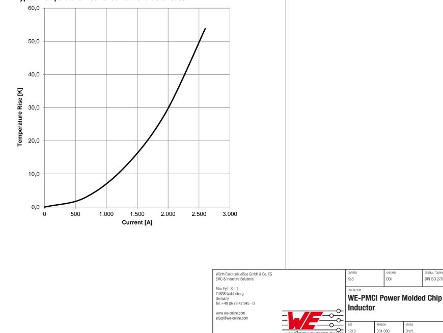
**Typical Temperature Rise vs. Current Characteristics:**
