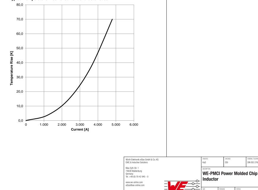
**Typical Temperature Rise vs. Current Characteristics:**
