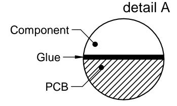
Customer to glue component on PC Board to ensure mechanical stability
