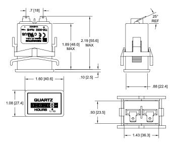
Panel Opening: 1.45" X 0.95" [36.8 X 24.1] Maximum Panel Thickness: 0.03 to 0.63 [0.76 to 16.00]
