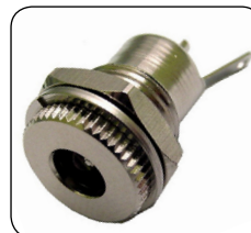
• 30-377 (Japan) • 30-377T (Taiwan) 2.1mm chassis mount coax power jack. Mounts 7/16" dia. hole.
