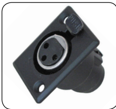
• 30-523-BK (3 Pin Black) • 30-523-SL (3 Pin Silver) • 30-523-SL-4 (4 Pin) • 30-523-SL-5 (5 Pin) XLR Female chassis jack. Mounts in 15/16" hole.
