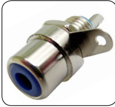
• 30-428-COLOR (Nickel Plated) • 30-428G-COLOR (Gold Plated) RCA Audio Jack with hex nut and solder lug. Mounts in 1/4" hole. AVAILABLE COLORS: BK, BU, GN, OR, RD, WH & YL
