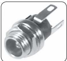
• 30-310 (2.1mm) • 30-311 (2.5mm) Chassis mount coax power jack. Mounts in 5/16" hole. N/C switch.
