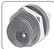
• 30-314 (2.1mm) • 30-315 (2.5mm) Chassis mount coax power jack. Mounts in 1/2" hole. N/C switch.
