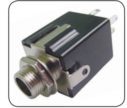
30-385 1/4" Stereo Audio Jack. with DPDT normally closed and normally open circuits.
