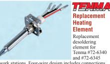
rework stations. Four-wire design includes connections for 24V, 48W element and integral temperature sensor. Ideal for replacing damaged elements, or upgrading older to accept the new, shorter length nozzles. Includes 2.0mm nozzle.
