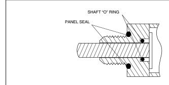
The shaft is sealed by an O-ring inside the bushing. The panel is sealed by an O-ring at the base of the bushing.
