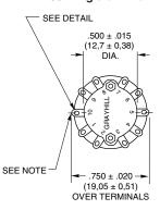
Note: Common location for a single pole per deck switch. For common location on multipole switches see circuit diagrams.
