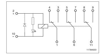
Figure 3. RMOB-JR-2 Relay Base Block Diagram
