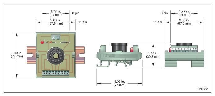
Figure 2. RMOB-JR-2 Relay Base Dimensions
