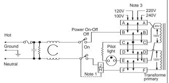
Note 1: Jumper required if only SPST power switch is used.
