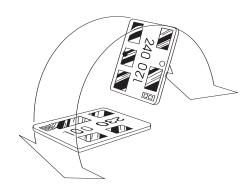
Open cover door and rotate fuse-pull lever to left. Select operating voltage by orienting voltage selection card, desired voltage on top left side. Push card firmly into module slot. Rotate fuse-pull lever back into normal position and re-insert fuse into holders. Use caution in selecting correct fuse value.
