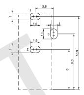
General tolerance  $\pm 0.05$  Do not use shunt terminal for power supply. Purpose of terminals 2 &~3 is only plug in / plug out detection
