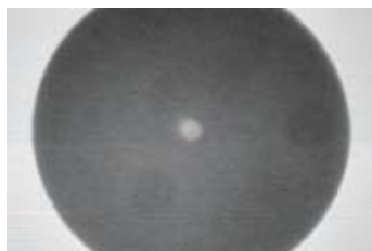
Ceramic Connector Cleaned with Novec Contact Cleaner
