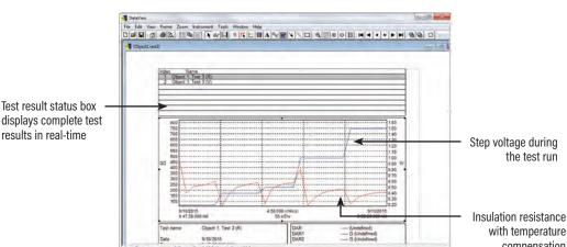
Test Summery | Object 1, Test 3 (R) | Object 2, Test 3 (V) | Run test and display text and graphical results from one dialog box. Model 5070 also displays step voltage.
