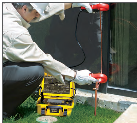
The Model 6471 provides a fast and easy way to measure the value of the earth/ground using the 2 Clamp method (no auxiliary rods needed).
