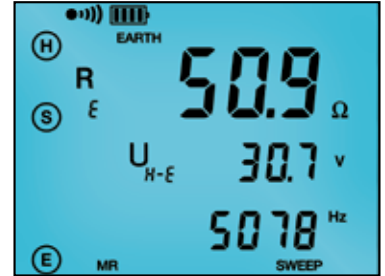
The 3-Point Fall-of-Potential test displays test lead connection, grounding rod resistance and test electrode resistances.
