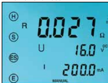
The 4-Point Bond test shows lead connections, bond resistance test results, test voltage and current.
