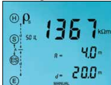
The Schlumberger test displays test lead connection, soil resistivity ( \rho ) test results and electrode spacing.
