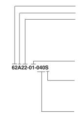
Style: A = 1/2" package, 5.0 Vdc Input, D = high torque w/5.0 Vdc input, V = 3.3 Vdc input
