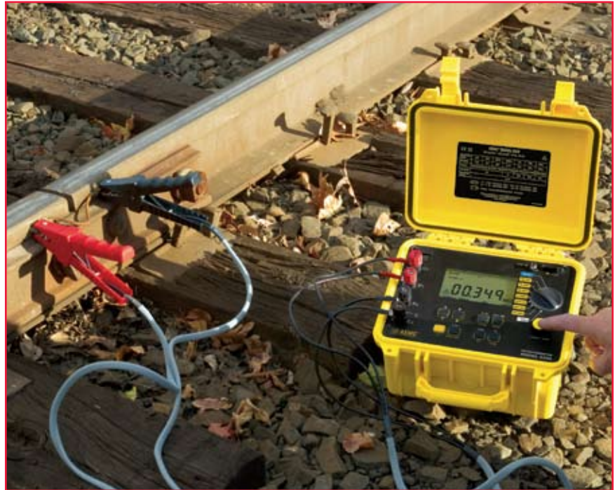
Verifying rail bonds with the Model 6250
